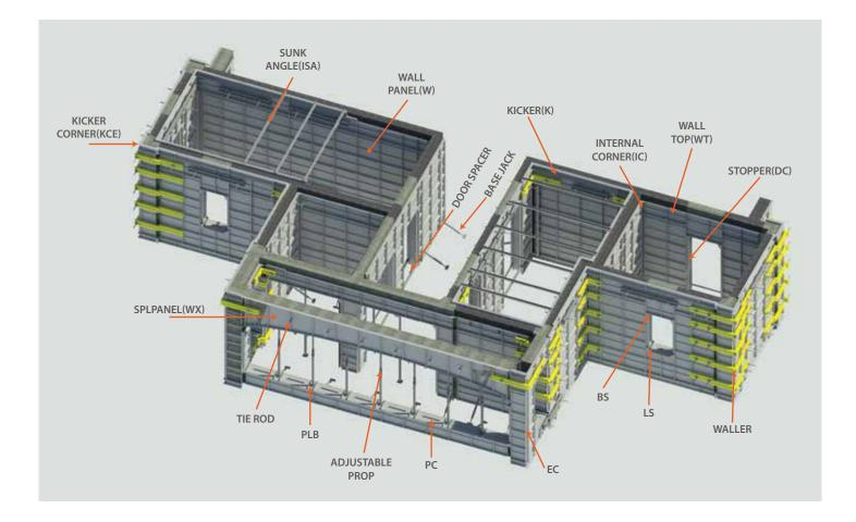
We create 3D designs of formwork in Revit for all our projects to provide our customers with a clearer understanding. This enables them to perform a complete walkthrough of the assembly prior to installation, helping to identify any potential mistakes or missing components. This approach prevents delays caused by missing items on-site.
